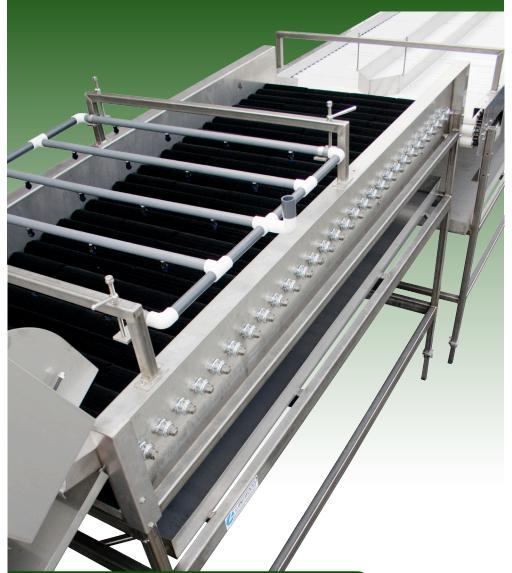
Includes a stainless steel drain pan to collect any excess water beneath the Brusher Bed
