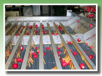
Radishes are conveyed onto the detailer bed where they are washed and dewatered. Radishes are conveyed through a series of flaps to a specially-designed knife that cuts the tail off of the radish without damaging it. The radish tails fall onto a conveyor underneath the detailing bed, where they are removed by your choice of a water-flush system or a trash conveyor.
