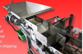
Our Volumetric Clamshell Filler for Grape & Cherry Tomatoes includes the industry's most effective **no-bridge hopper system**, designed specifically to allow small tomatoes to fill containers without bridging or clogging the filling area.
