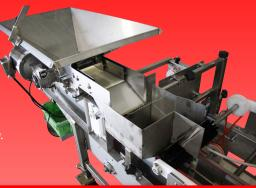
Our Volumetric Clamshell Filler for Grape & Cherry Tomatoes includes the industry's most effective **no-bridge hopper system**, designed specifically to allow small tomatoes to fill containers without bridging or clogging the filling area.
