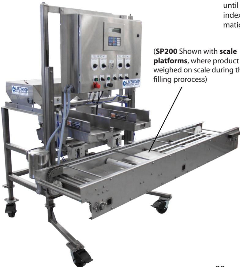
(SP200 Shown with **scale platforms**, where product is weighed on scale during the filling process)
