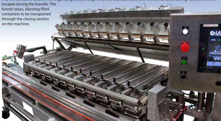
^ Tilt belt and feeder trays easily flip up for quick access and cleaning
