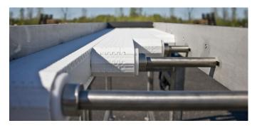
Multiple staggered belts allow product to discharge from the stagger belt evenly onto conveyors below
