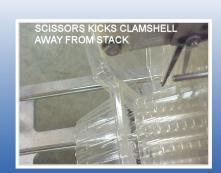
(Single Lane Scissors Denester, shown in-line with a Single Lane Volumetric Clamshell Filler and a Dual Level Pack off Conveyor)
